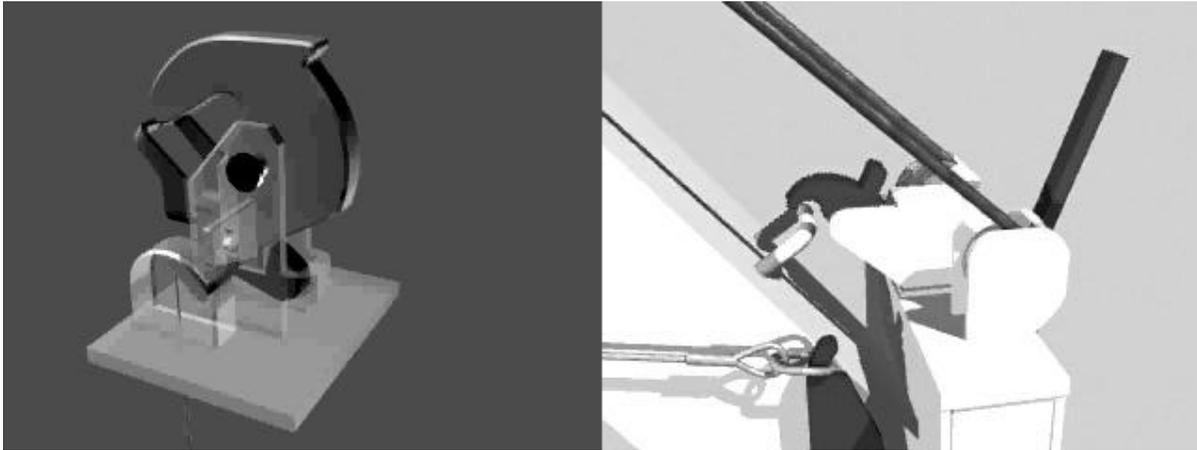
Figure 4. Shows a hook release mechanism and davit activating gear. The interface incorporates interactivity in a near authentic environment.
