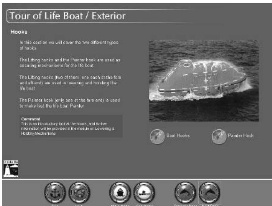
Figure 3. Shows the section dealing with boat hooks and painter hooks
