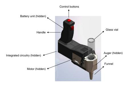
Fig 1: Handheld solid dispenser prototype.
